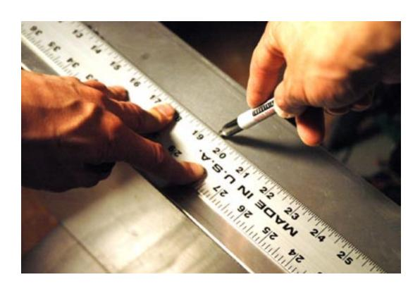
One way of marking the front is to place a line centred horizontally across the face of the case.
