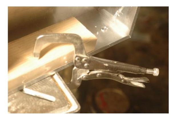
A small piece of 2x4 will help protect the case from Indentation and also give the clamps a good surface to bite into.
